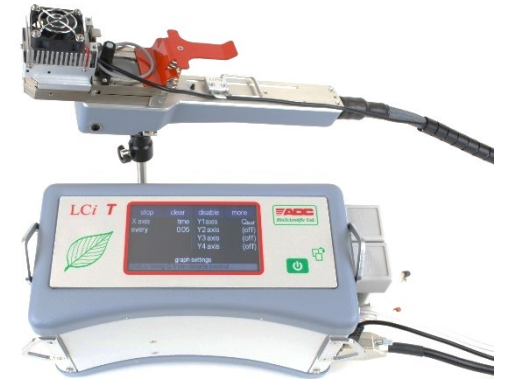
Infra-red gas exchange system
